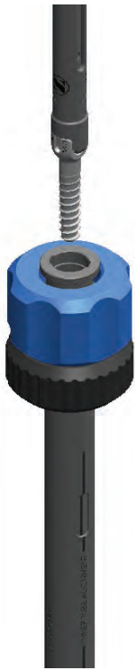
Figure 37 Screw insertion through ATO
