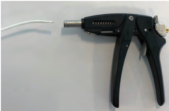
Figure 68 Cord insertion through tensioner
