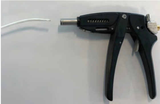
Figure 47 Cord insertion through tensioner
