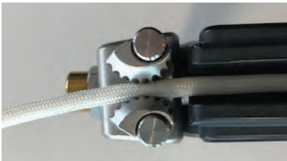
Figure 48 Capture cord with tensioner rack cleats
